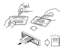
Clean the heads after every 10 hours of use using a wet-type head cleaning tape (available at an audio store).
